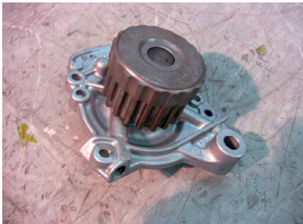
Figure 2.165 Water pump drive gear (cam belt)
